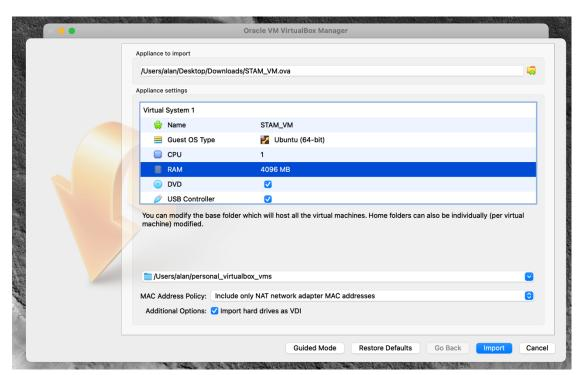
3d) If necessary, Raise or lower the amount of RAM and number of CPUs selected for the VM. NOTE: The TA set their CPUs to 3 after having long loading times
